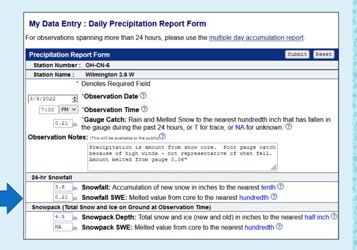
4) Snowpack Depth—measured to the nearest half inch and measured from ground using snow stick. This includes both new snow and snow that was already there.
