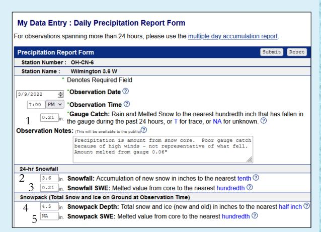
1) Gauge Catch— measured to the nearest hundredth and measured with your rain gauge with the goal of determining how much liquid is in the snow (or mix of precipitation)
