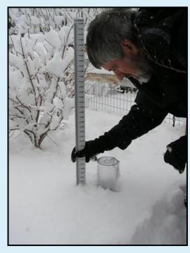
Note that we never measure the depth of the snow in the rain gauge itself. Any frozen precipitation in the rain gauge must first be melted, then measured.
