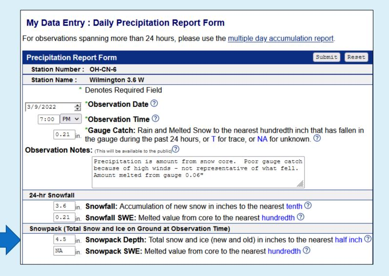
5) Snowpack SWE(optional, but encouraged...especially on Mondays) – measured to the nearest hundredth and measured with gauge. This helps determine how much liquid is in the new and old
