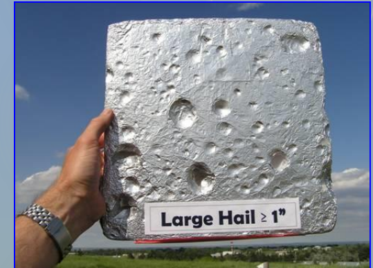
Aluminum foil-wrapped Styrofoam hail pads
