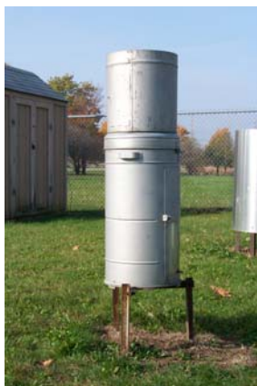
Weighing bucket rain gauge
