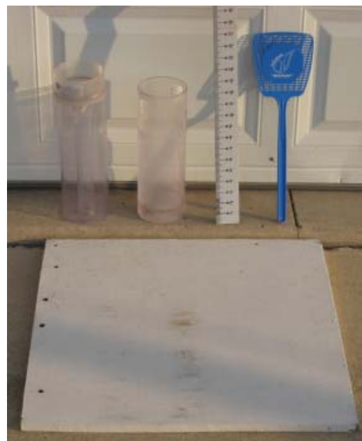
Winter precipitation measuring equipment: a rain gauge, extra outer cylinder, snow ruler, snow swatter, and snowboard.
