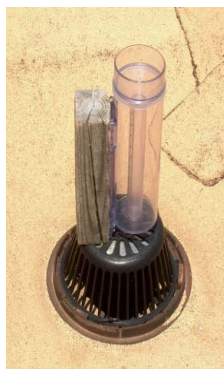
The IL-CK-36 rain gauge is mounted on a roof drain cover.
