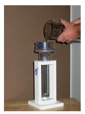
The MTS provides solid support for both the inner tube and the funnel, allowing you to easily control pouring of water from the four-inch outer tube.
