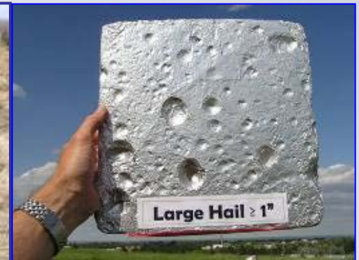
Aluminum foil-wrapped Styrofoam hail pads
