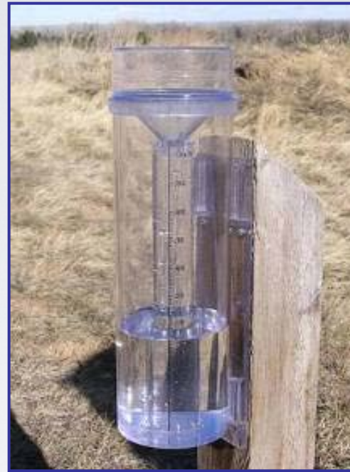
4-inch diameter high capacity rain gauges
