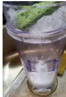
WHILE THE SOAP, WATER AND SPONGE ARE IN USE, CLEAN THE FUNNEL AND OUTER CYLINDER.
