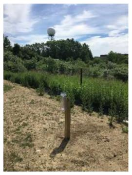
It looks like an ordinary 4" diameter rain gauge on a post. That Doppler Radar antenna in the background makes the location unique. The absence of grass surrounding the gauge does indicate some recent disturbance of the land.
