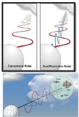
There are several benefits of the Dual-Pol radar. First, it improves accuracy of precipitation estimates, leading to better flash flood detection. Next, it has the ability to discern between heavy rain, hail, snow, and sleet. It also improves identification of non-meteorological echoes (e.g. ground clutter, birds, and even tornado debris). Lastly, it helps in the detection of aircraft icing conditions by having the ability to identify the location of the melting layer (e.g. bright band).
