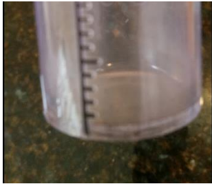
DIRT ON THE BOTTOM OF THE INNER CYLINDER
