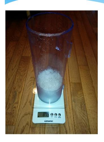
If you are weighing daily snowfall in your 4 inch precipitation gauge or from a snow core simply place the gauge with contents on your scale and measure the weight in grams:
