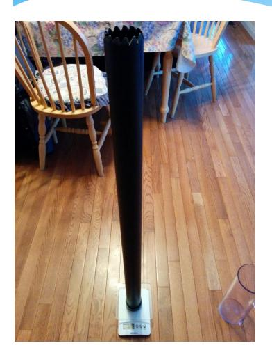
Bring your **2 inch** snow tube inside and place it on the scale. Be sure to first remove any snow or moisture on the outside of the tube:
